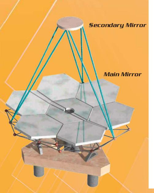
A new concepts of telescopes with adaptive mirrors is now becoming real, Similar smaller size concepts are being developed. Nanomotion participate is such a program and enables solution for main mirror segment alignment. It requires high accuracy (nm level), 6 degree of freedom in small size, light weight and zero power consumption when holding position.
